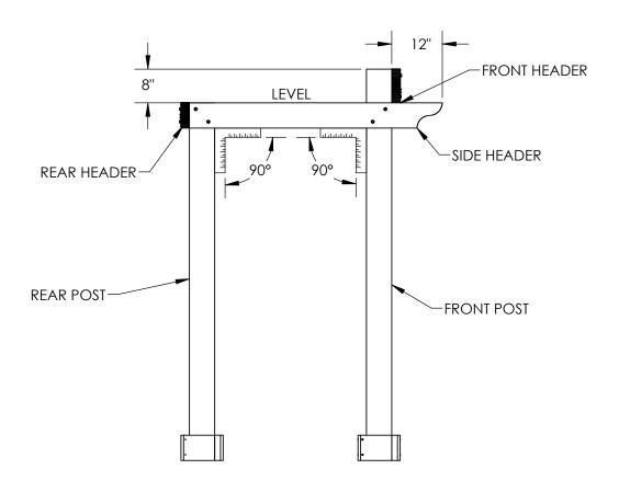
7.2 - SECURE USING 4" TIMBERLOCK SCREWS AND CAP NUTS AS SHOWN BELOW.
