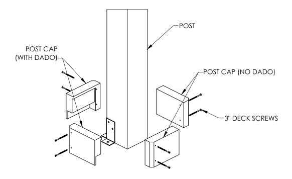
3.2 - FASTEN TO CORNER POSTS USING PROVIDED WOOD SCREWS.
