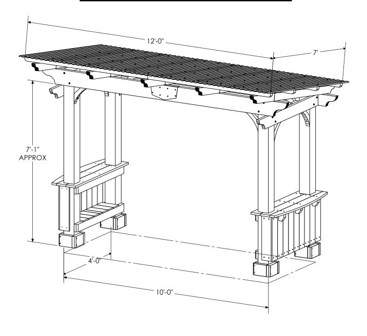
TOTAL HEIGHT: 8'-5" FRONT HEAD CLEARANCE: 7'-1" REAR HEAD CLEARANCE: 6'-7"
