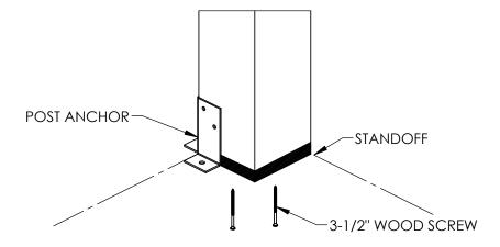
2.2 - IF POST ANCHOR IS TO CLOSE TO CONCRETE SLAB EDGE, POST ANCHOR CAN BE MOVED TO INSIDE CORNER.
