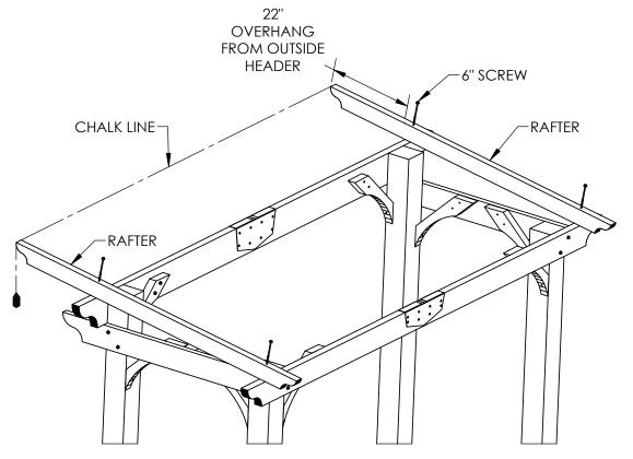
9.1 - LAY REMAINING RAFTERS AND SECURE WITH 6" SCREWS BY GOING DOWN THROUGH THE PREDRILLED HOLE IN RAFTER AND SECURING TO THE FRONT AND REAR HEADER AS SHOWN BELOW.
