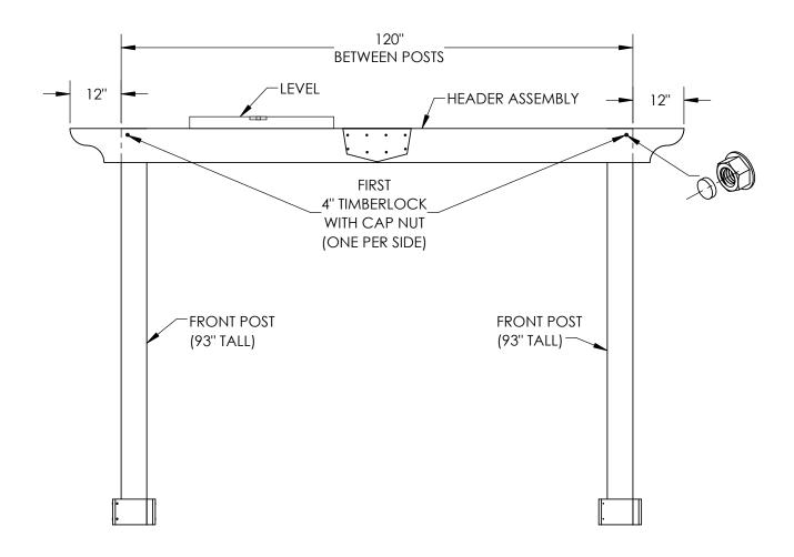
5.2 - CHECK POST TO HEADER CONNECTION WITH A SQUARE. INSTALL SECOND TIMBERLOCK SCREWS AND CAP NUTS TO EACH END AS SHOWN BELOW.
